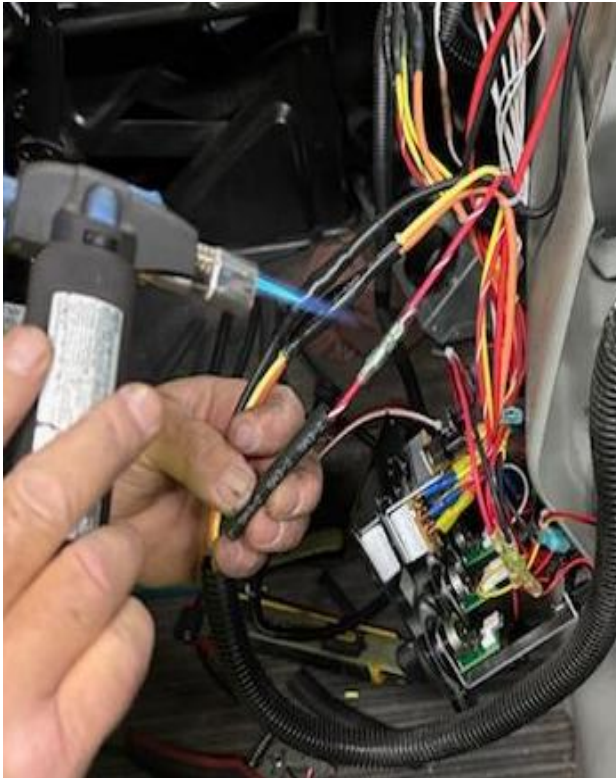
Figure 9 – Solder filled butt connectors and heat-shrink tubing.
