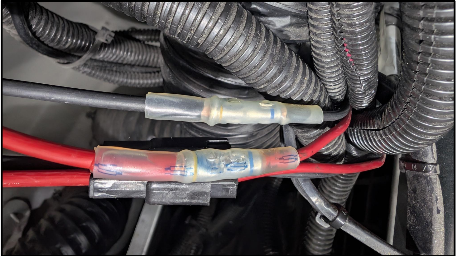
Figure 10 – Double size butt splice connectors.
